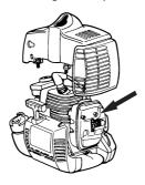
Some mufflers are equipped with a special spark arrestor mesh. If your machine has this type of muffler, you should clean the mesh at least once a week. This is best done with a wire brush. On mufflers without a catalytic converter the mesh should be cleaned weekly, or replaced if necessary. On mufflers fitted with a catalytic converter the mesh should be checked, and if necessary cleaned, monthly. If the mesh is damaged it should be replaced.
